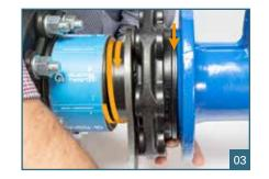
Bring the profile gasket into the correct position on the fitting flange and adjust the HP flange of the QUICK-TWIST with a turning movement until the profile gasket is held in place.
