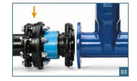
First, install the fixed flange side (special flange VP) of the QUICK-TWIST to the counterflange. A profile gasket is not required for this, as an O-ring seal is provided.
