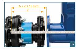
Make sure that the maximum adjustment path of the QUICK-TWIST (+ 15 mm as standard) is sufficient to bridge the installation gap and create the flange connection to the fitting. Also take into account the thickness of the profile gasket.
