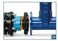
Set back the HP flange of the QUICK-TWIST with a turning movement until you have enough space to remove the fitting. Remove the profile gasket.
