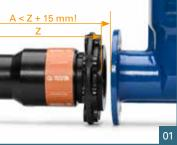
Make sure that the maximum adjustment path of the QUICK-TWIST (+ 15 mm as standard) is sufficient to bridge the installation gap and create the flange connection to the fitting. Also take into account the thickness of the profile gasket.
